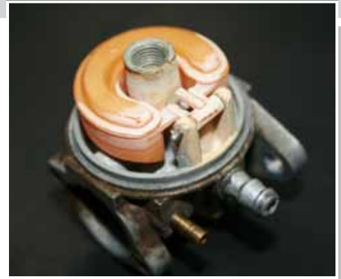
Corrosion inside carburetor
