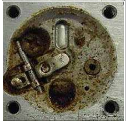
Carburetor damage from stale fuel
