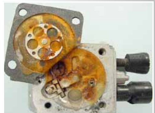
Corrosion from water inside carburetor
